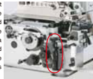
Differential-feed micro-adjustment mechanism
