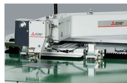
Easy maintenance! New arm-shaped, glass epoxy slide plate
